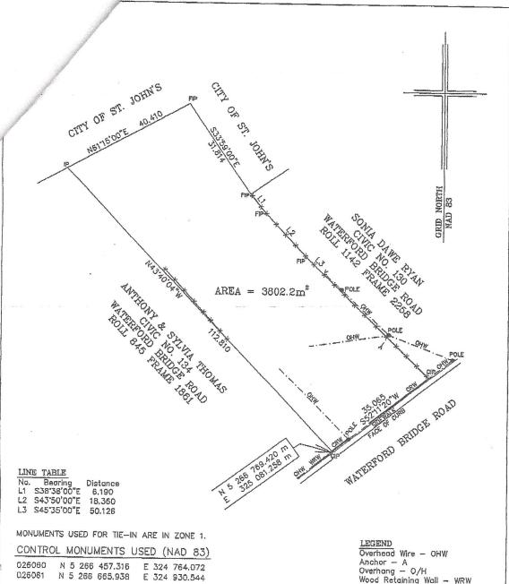
SCALE FACTOR OF 0.999900 USED FOR THE COMPUTATIONS OF STARTING CO-ORDINATES ALL OTHER GROUND DISTANCES ARE HORIZONTAL GROUND DISTANCES.
